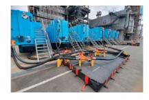
Mark Orr talked about the tankers and bulked storage highlighting that they are ideal for small incidents. He also presented the bladder tankers explaining that they are useful and can cluster them together so vac tanker feed the storage farm. He underlined that the only disadvantage of the bladder tanker is that it needs much space.
